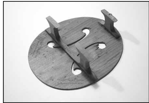
Fig 3. The Virzi Tone Producer is a thin piece of very-wide grain spruce that was suspended by three feet. This one was removed from an original Loar-signed F5 mandolin.
